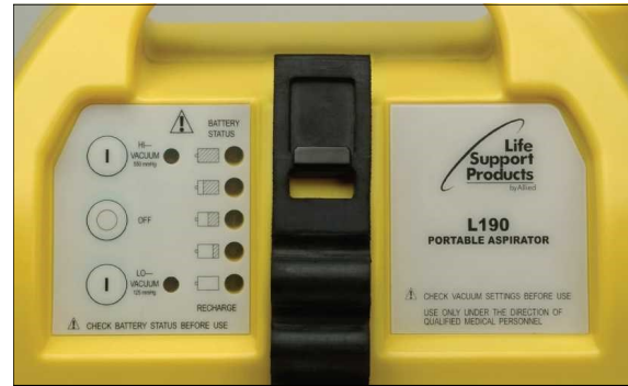
L190 High and low vacuum switches to select pre-set 550 mm Hg or 125 mm Hg vacuum modes.
